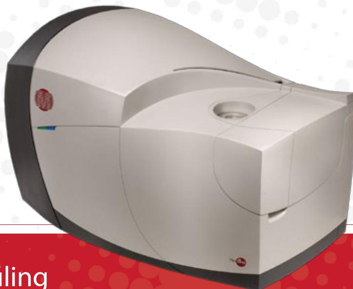
MiniSIMS imaging & profiling rapidly analyse multi-layer coatings for continuity, composition and thickness.
