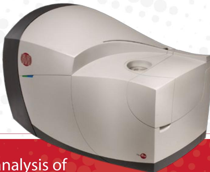
MiniSIMS mass spectral analysis of surfaces can be used to monitor surface treatments with sub-monolayer sensitivity.
