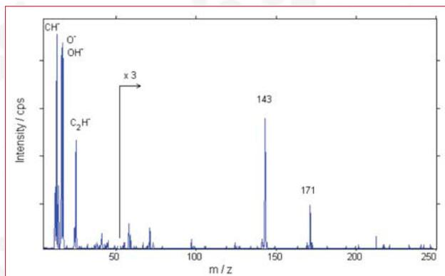
Figure (1) SURFACE SPECTRUM REVEALING PRESENCE OF A CUTTING FLUID
