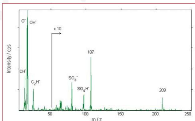
Figure (3) SURFACE SPECTRUM REVEALING PRESENCE OF A METAL CLEANING AGENT
