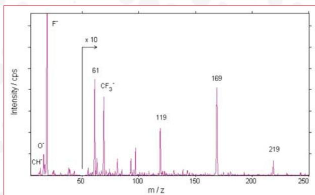
Figure (2) SURFACE SPECTRUM REVEALING PRESENCE OF A LUBRICANT ADDITIVE
