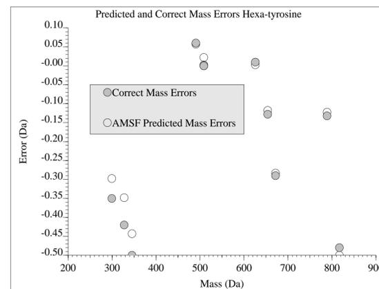
Figure 2 Mass Assignment Errors and AMSF Assignment Errors Showing the Correlation between Theoretical Mass Assignment Error and AMSF Predicted Errors in the Context of Instrumental Error
